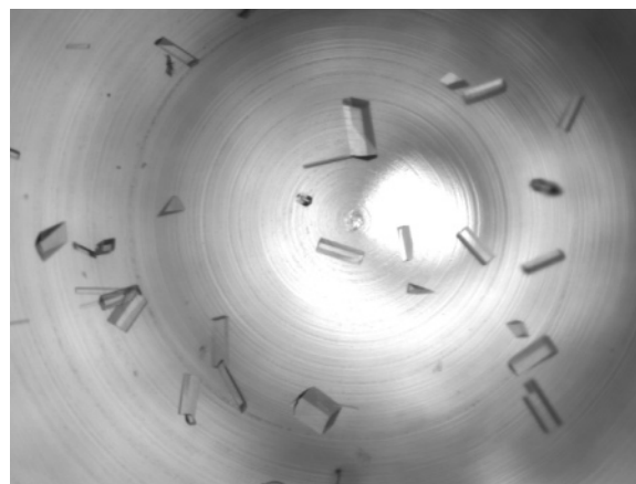
Figure 6. Example image of lysozyme crystals grown using the stepwise NaSCN concentration profile shown in Figure 5. The image was taken from a dialysis button in cell 3 at the conclusion of the experiment (223 h). The crystallizing solution consisted of 3.21 mg/mL lysozyme in 50 mM acetate buffer pH 4.6 at approximately 20 °C.
